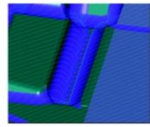
Fillets can also be specified to have a different radius to the diameter and this can be useful if 3-axis machining with carbide-insert button cutters.
