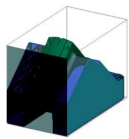
difference between a remaining material stock model and the finished component.
