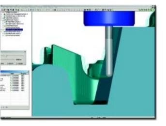
In operation, a set of toolpath passes can be created without a toolholder. These passes can then be edited to a toolholder whereby the minimum tool length can be established.
