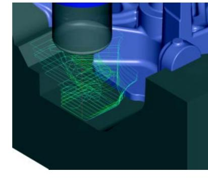
Cutter contact is maintained as much as possible to avoid the reduction of tool life.
