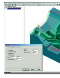
With rapid moves, the default is for shortestroute rapids which look ahead at the surfaces/stock model and take a "racing-line" approach to the next cut move.
