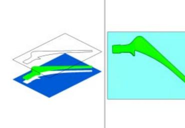
If planar holes are located at a vector in space, these can also be filled, by specifying an AB rotation for the boundary used to constrain the planar patch.
