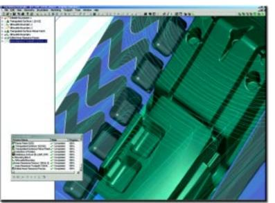
If both a helix entry or a profile-ramp entry would leave material under the effective cutting diameter of the cutter, which might result in the cutter being damaged as it drops deeper in Z, *machining* **STRATEGIST** discards this part of the toolpath, to be picked up later by a rest-material re-machining operation.
